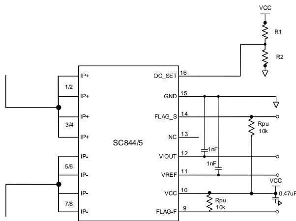
**20kA/8us Over Current surge, High Accuracy Current Sensor with Adjustable Over Current Fault Detection Current Sensor IC**
