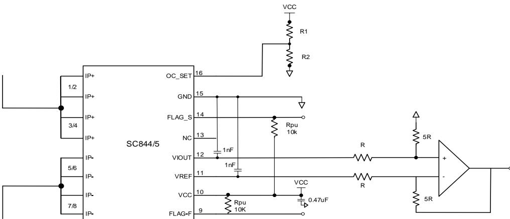
**20kA/8us Over Current surge, High Accuracy Current Sensor with Adjustable Over Current Fault Detection Current Sensor IC**
