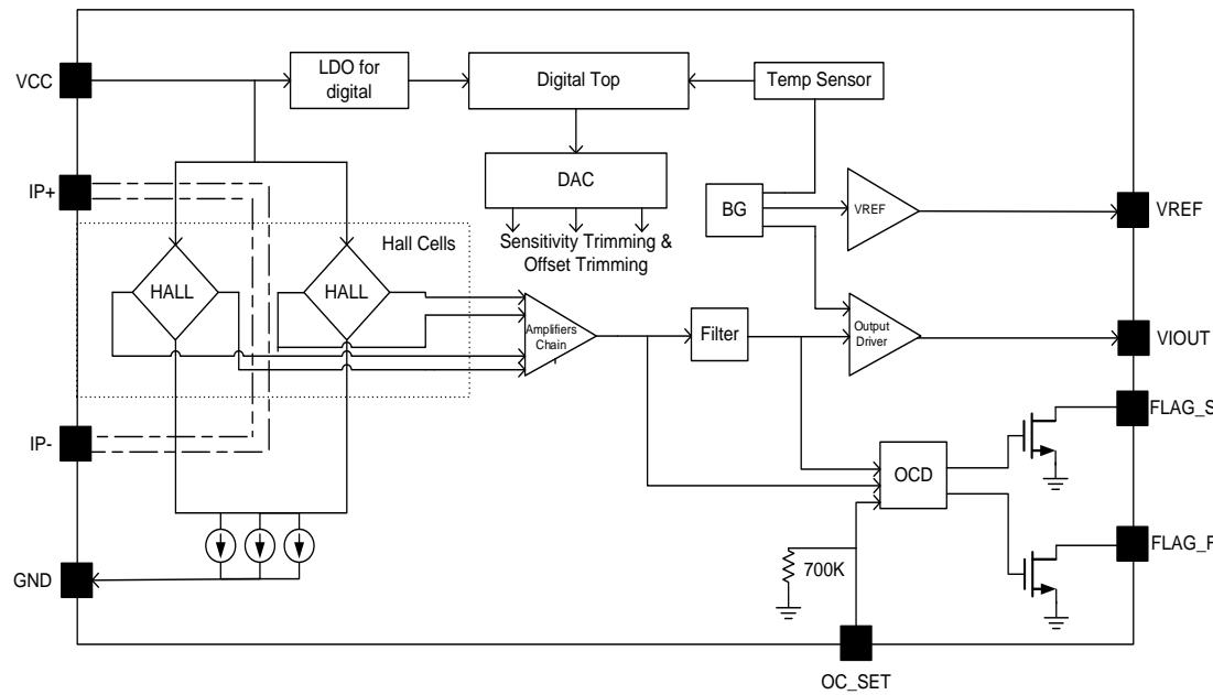
**20kA/8us Over Current surge, High Accuracy Current Sensor with Adjustable Over Current Fault Detection Current Sensor IC**
