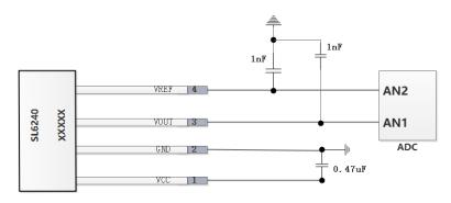
VREF is the output terminal when selecting 2.5V function.
